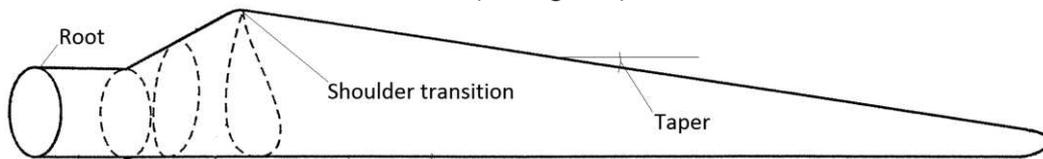
**Figure 1** Typical LGVs in turbine blades such as taper (smooth) and the 'shoulder transition' (non-smooth).
