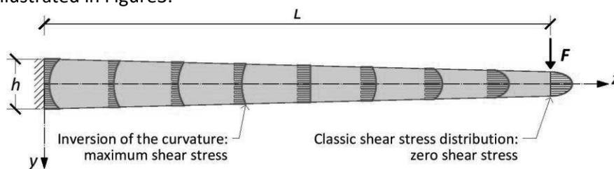
**Figure 3** Shear stress distributions (red hatch) in a tapered beam differ in different cross-sections and can be significantly at variance with prismatic cases depending on the taper angle and the loading conditions.
