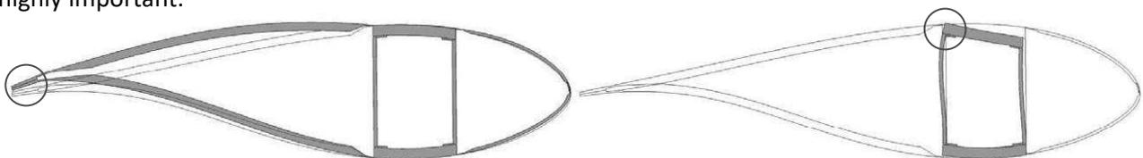
**Figure 2** Geometrically non-linear cross-section deformations (solid grey) severely affects the trailing edge joint (left) and web-to-cap joint (right) by inducing prying-forces into blade components having the tendency to rip bond lines apart.
